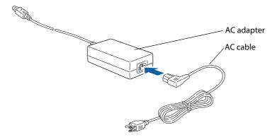
Insert the connector of the power supply cable onto the power supply connector (stamped **24V**).
