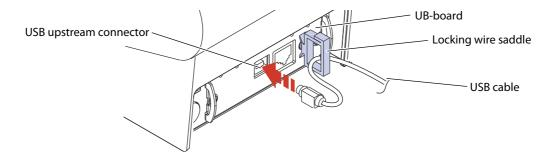
**3** Connect the USB cable from the host computer to the USB upstream connector.
