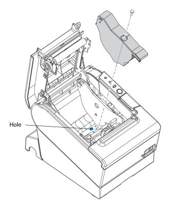
Tighten the enclosed screw to fix the roll paper guide.
